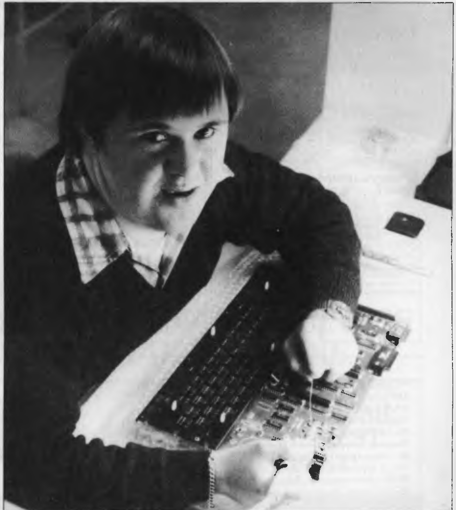
Fixing keyswitches to the PC board, Charles Tame shows he can handle a soldering iron with skill and concentration.
