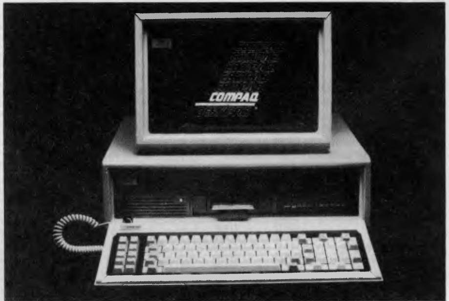
The Compaq Deskpro family consists of the first high-performance 16-bit desktop personal computers to run the Intel 8086 microprocessor while maintaining compatibility with the IBM-PC and XT.
