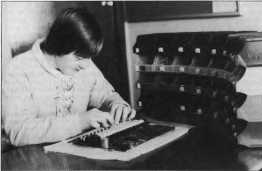
Ruth Hutton attaches keytops to switches. The keys are kept in trays which follow the order of the QWERTY keyboard layout.
