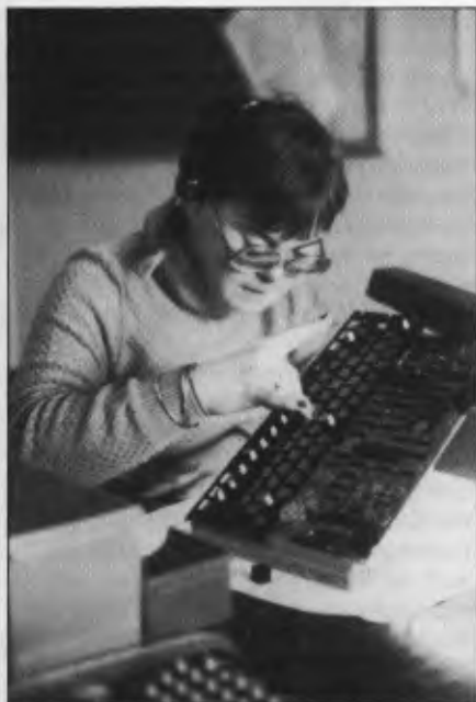
Debbie Roberts places keyswitches, a task which requires careful alignment of pins on the switch with punched holes on the printed circuit board.
